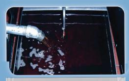
DRAIN THE OIL FROM FRYER INTO THE FILTER PAN
