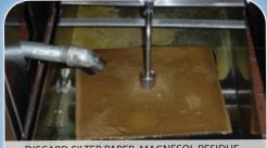
DISCARD FILTER PAPER, MAGNESOL RESIDUE AND CLEAN YOUR FILTER PAN TO ENSURE THAT IT IS READY FOR USE
