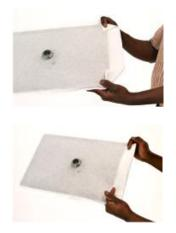
• Slide the filter clamps over the folded edge, with the folded side on top and the flat side on the bottom. Make sure the fold is at the top, toward the standpipe.
