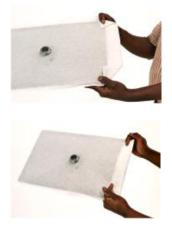
• Slide the filter clamps over the folded edge, with the folded side on top and the flat side on the bottom.
