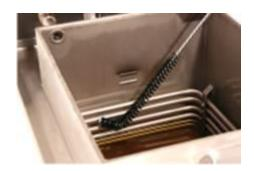
• Once all the oil has drained, clean the drain opening using a straight brush.
