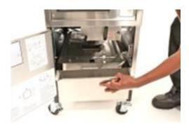
• Check that the cooker is level. The oil must be at an equal distance from the rim of the cook pot on all sides.
