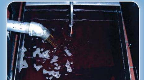
DRAIN THE OIL FROM FRYER INTO THE FILTER PAN
